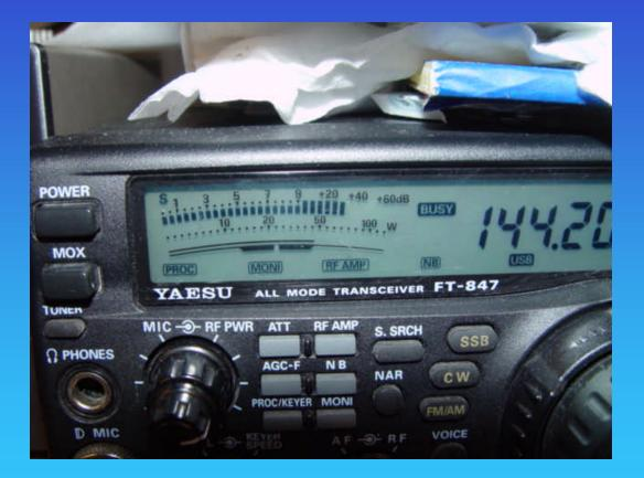
Make measurements with the noise source off then with the noise source on. The measured difference is the Y-factor. The Y-factor, combined with the actual ENR of your noise source provides you with the necessary information to calculate your noise figure of the system.
