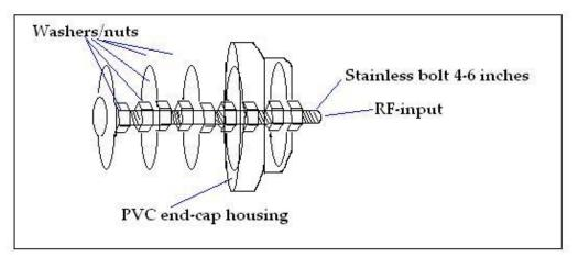
Fig. 1: IFA "Spaced-Washer Probe" Concept
