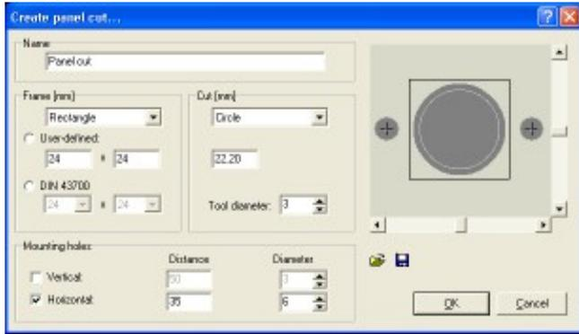
This function creates a group which contains the frame for the component dimensions and the cut for the component. Circles and rectangles are available as shapes for the frame and the cut. Mounting holes can be added if necessary. The distance of these holes is measured between the centres of the holes.
