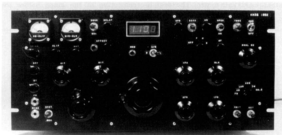
Fig 1—In my home-brew transceiver shown here, the AGC switch is labeled OFF-F-M-S. The SQUELCH (down) switch is part of the OPERATE (up) and STANDBY (center) switch, which is labeled merely OPER-SQ. The meters read signal level in dB and squelch integrator charge. Not shown here are the three separate transceiver front-end sections for MF/HF, 6 meters, and 2 meters.
