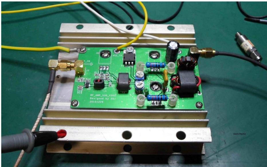
My completed amplifier undergoing bench tests
