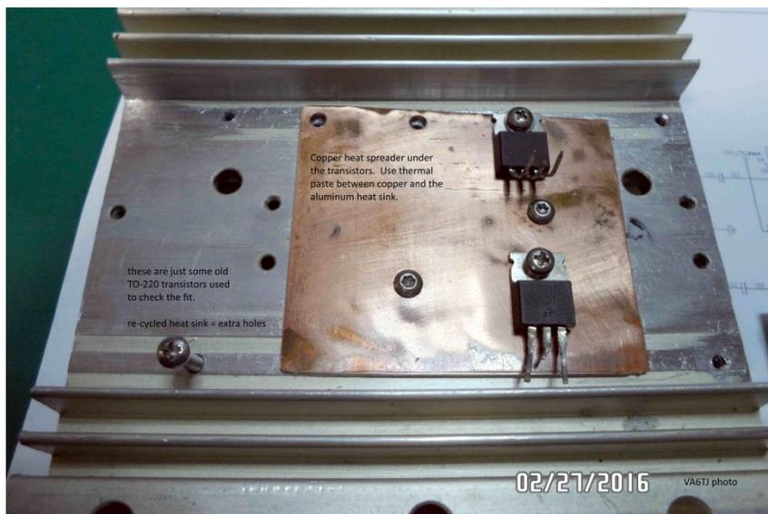
1. Drill holes in the heat sink corresponding to the position of the mounting holes in the TO220 Transistors (not the 7809 regulator), drill and tap holes for 3.0mm diameter screws. After drilling, clean the surface of the heat sink carefully, and don't leave any metal chips that could cause a short circuit. (If you use different hardware, e.g. 4-40 the drill size must be changed
