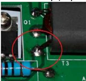
5. Open one side of the T3 transformer (The red circle shown the graphic below), and then connect the multimeter/ammeter between the pads for L1; make sure meter is at 10A range position. Adjust the potentiometer RV2 slowly anti-clockwise until the measured current is between 25 and 30mA. Make sure ammeter leads do not pass close to the input side of the board. (See my note below on using a resistor and voltmeter instead
