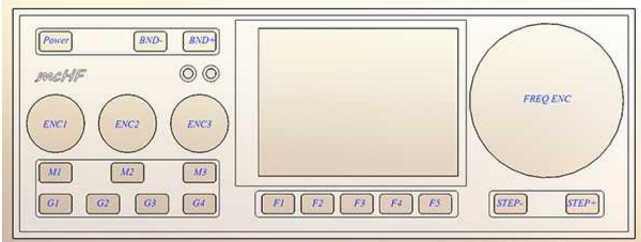
*Figure 1: Front panel controls of the mcHF transceiver*
